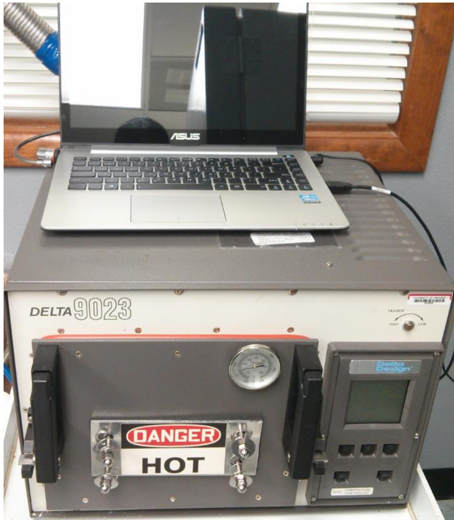
Figure 5.3: Thermal cycling furnace
