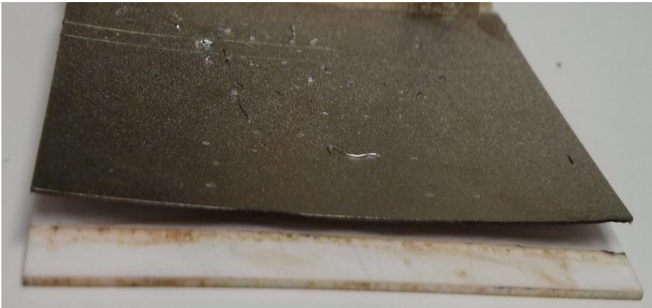
Figure 5.10. De-lamination of Copper layer from the Al 2 O 3 substrate.
