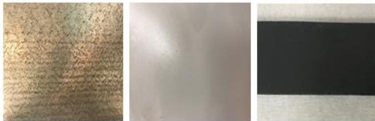
Figure 20: Translation test samples. Left: aluminum sheet with texture, middle: white painted aluminum sheet right: Rubber
