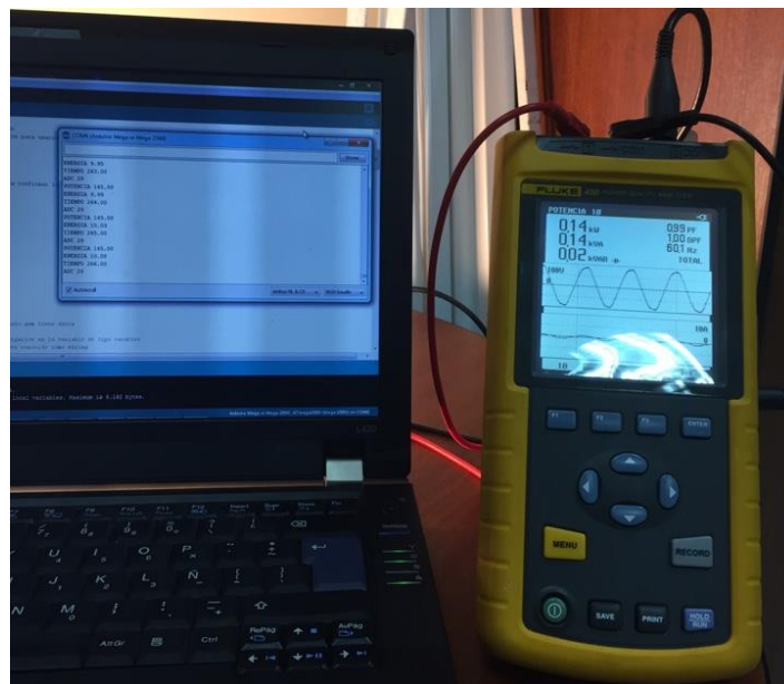
Figura III.17 Lecturas Arduino vs Fluke 43B
