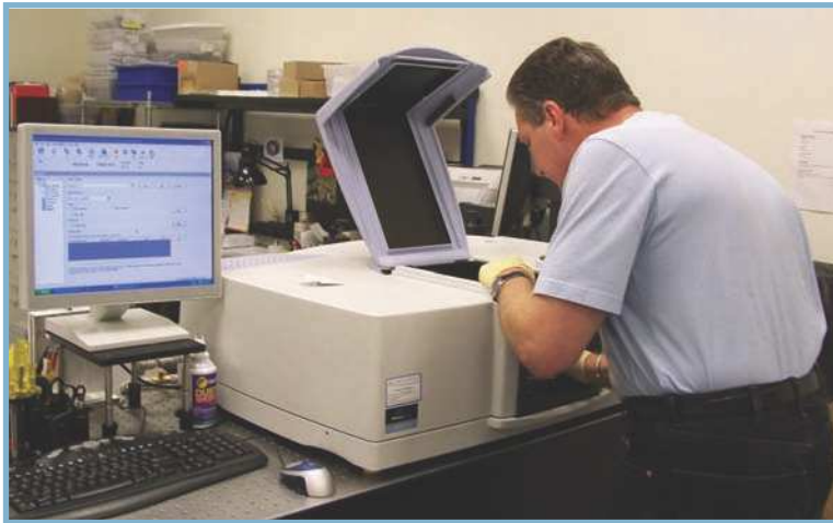
Operator testing filters on a spectrophotometer after a coating run. All Thorlabs filters undergo rigorous testing before being made available for sale.
