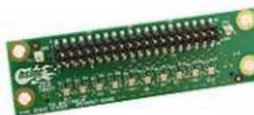
Figura 25 HSMC Port B (J9) – (Debug Header Shown)
