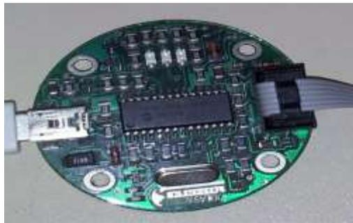
**Figura 15 Programador PIC (2012)**
