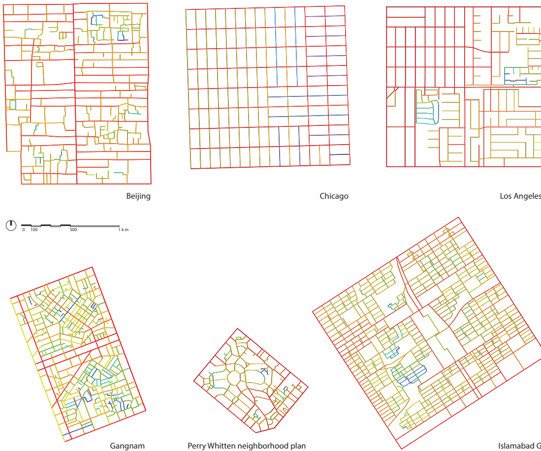
Figure 22 : Distribution of directional distances. Lower values in red, higher values in blue.
