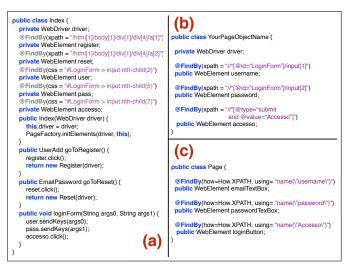
Fig. 2. Comparison between a Page Object generated by APOGEN and those of OHMAP and SWD Page Recorder for the login page in Fig. 1
