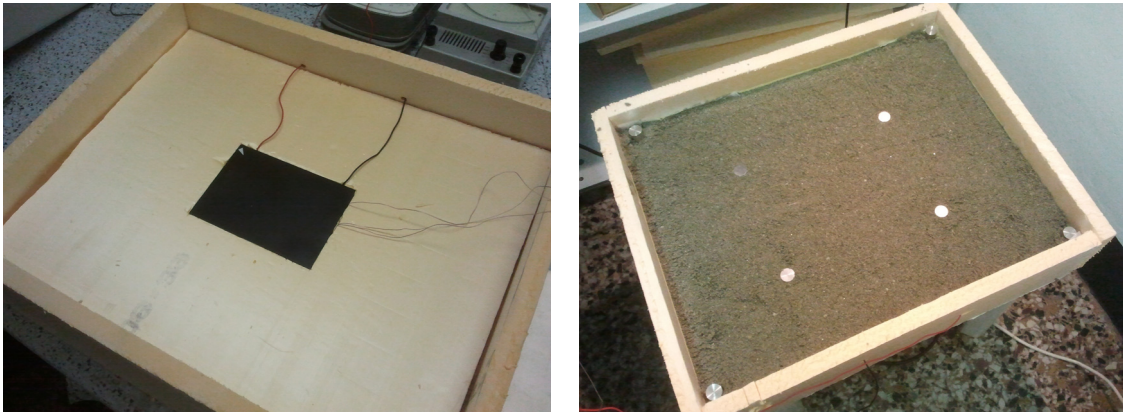
Figure 1. The container simulating a landfill with biogas production: the thermal source (left) and the covering sand layer (right).
