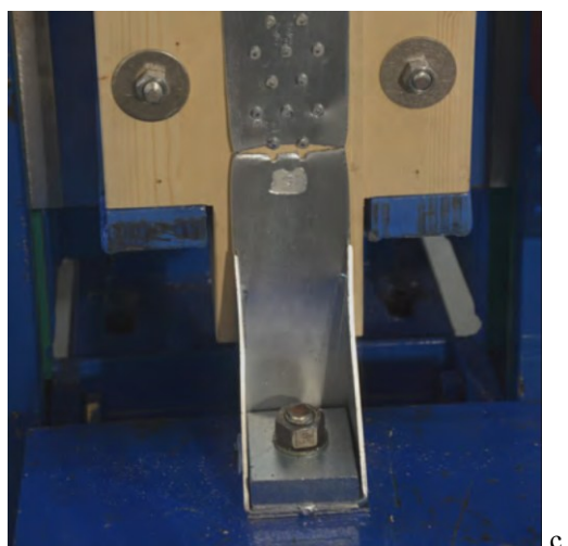
Figure 4.1. Inappropriate failure mechanisms at the connection level: (a) failure due to withdrawal of the nails connected to the floor panel; (b) failure due to pull-through of the anchoring bolt, and (c) tensile failure of the net cross-section of the metal flange (courtesy of CNR IVALSA and University of Trento, Italy).
