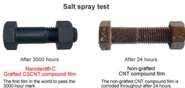
Figure 3.2. Example of a screw coated with Nanotect® and a normal screw upon corrosion with a salt spray ( http://www.takenaka-mfg.com/technologies/nanotect.html ).
