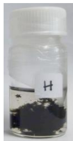
Figure 2.7. Aggregates of MWCNTs in ethanol ( 1 \text{ mg ml}^{-1} ).
