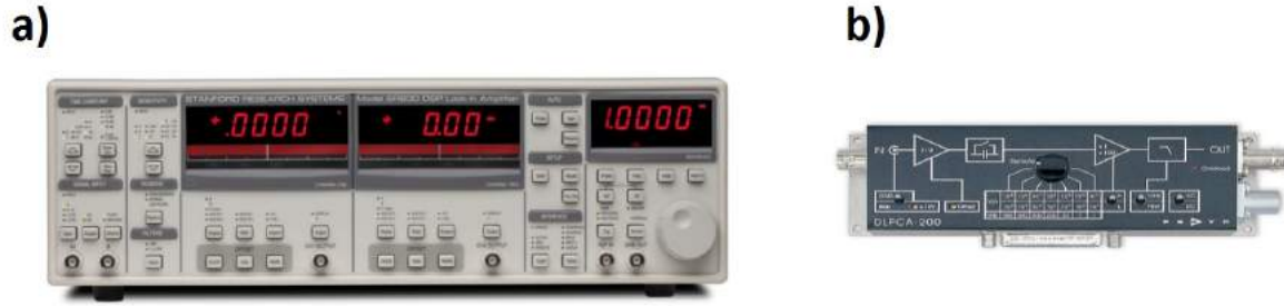
Figure 7: a) Front view of the lock-in amplifier, model SR830 by Stanford Research Systems. The tool can be used in the output frequency and voltage ranges ranging from 1 mHz to 102 kHz and from 4mV to 5V (error 1%), respectively. b) Picture of the trans-resistance amplifier DLPCA 200 by Femto. The amplifier can be used both for DC and AC current-signal and the amplification factor can be tuned in a very broad range, from 10^3 to 10^{11} V/A.
