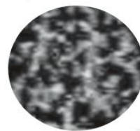
Figure 3.11: example of a speckle pattern produced by light scattering. (From ref. 32)
