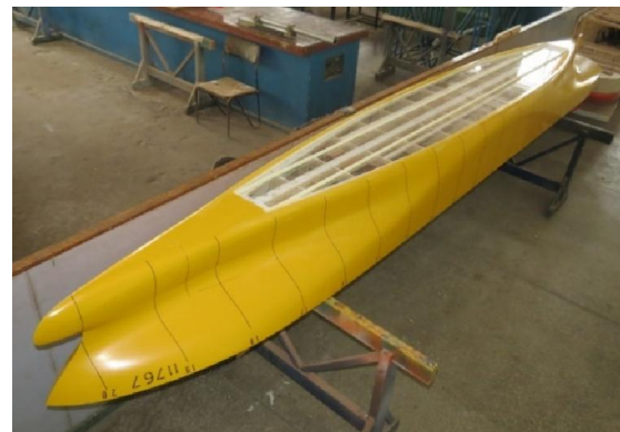
Fig. 2 Containership model with the recess.
