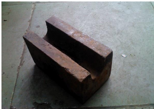
Fig. 3.1: SGCI test block after sand mold casting.
