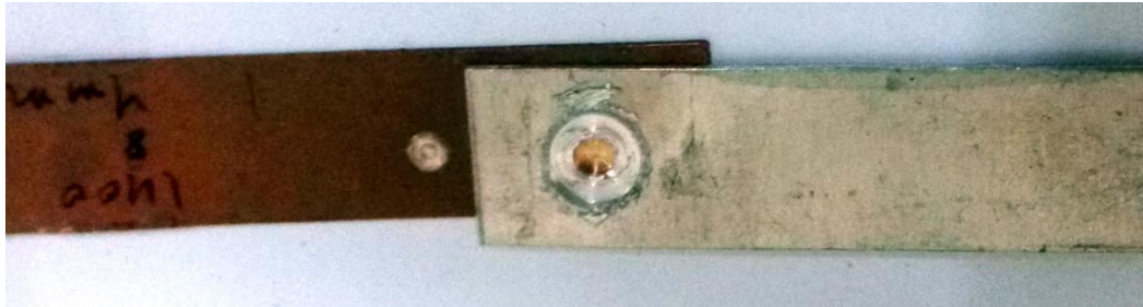
Figure 5.1 Weld generated between dissimilar metals
