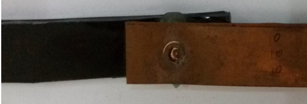
Figure 6.1 Work piece and the weld generated
