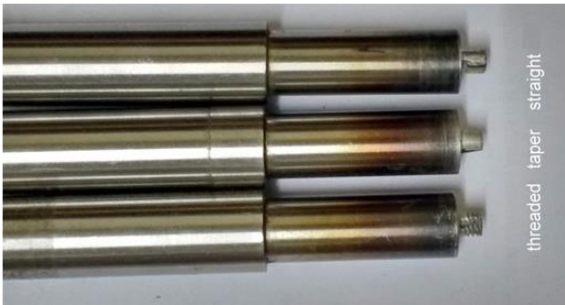
Figure 3.4 FSW tools used for the experimentation
