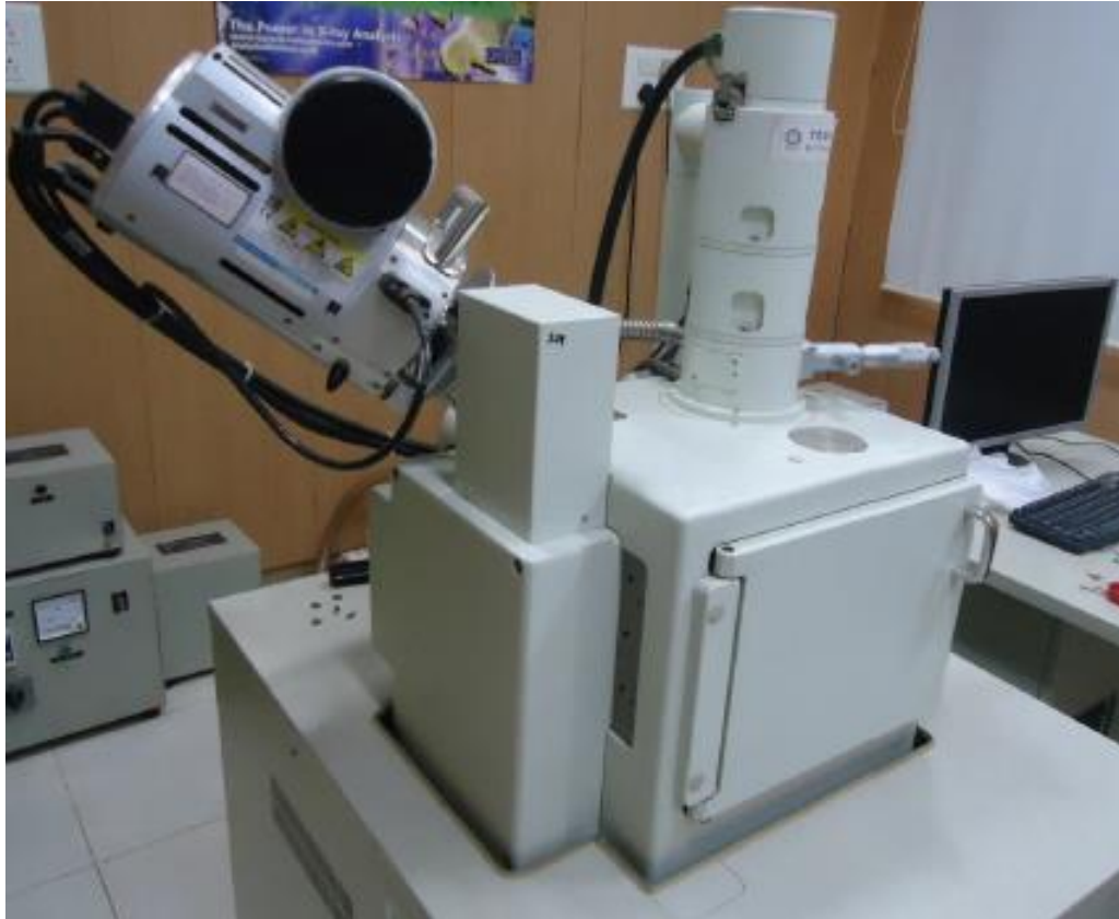
Figure 3.2 Scanning electron microscopy-Energy Dispersive Spectroscopy Instrument (Model JEOL JSM-6048LV)
