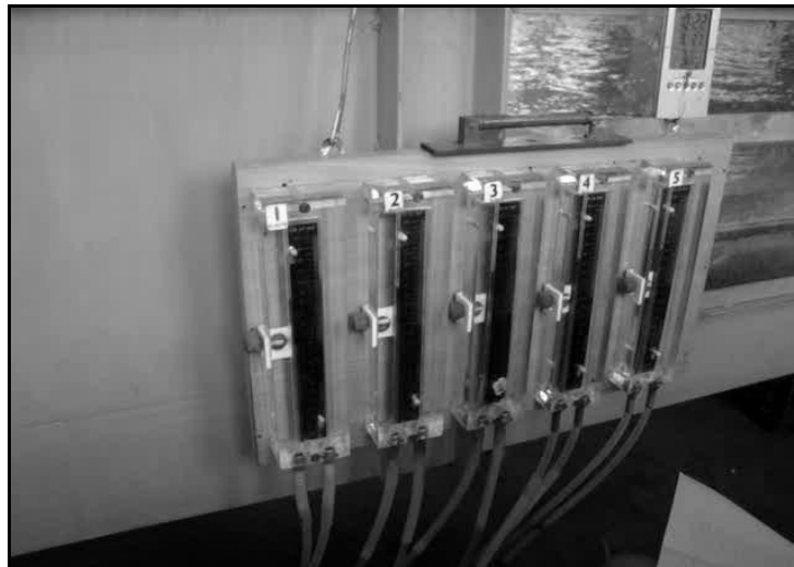
Figure 3.7: Series of Manometers, Spirit Level &amp; Stop Watch Hung Outside the Flume
