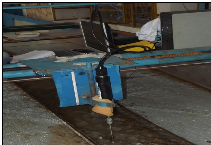
Figure 3.8: Micro-ADV Fitted to the Holder
