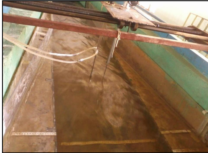
Figure 3.3: Micro-Pitot Tube Fitted to the Holder
