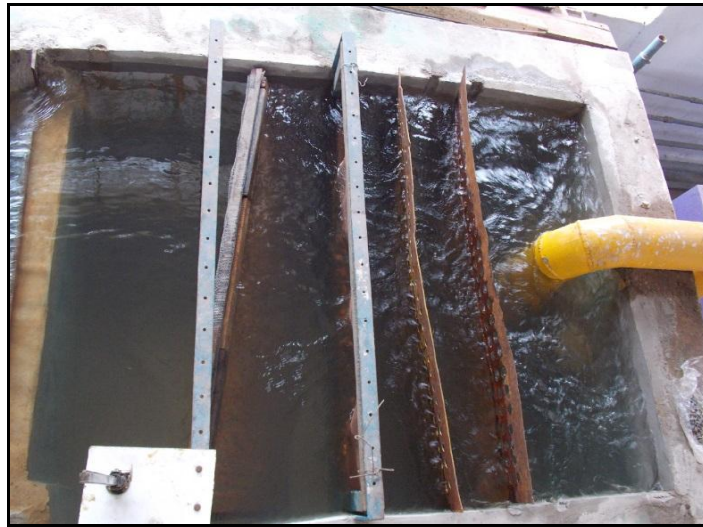
Figure 3.2: Stilling Chamber, Flow Straightener & Point Gauge In U/S Section of Flume
