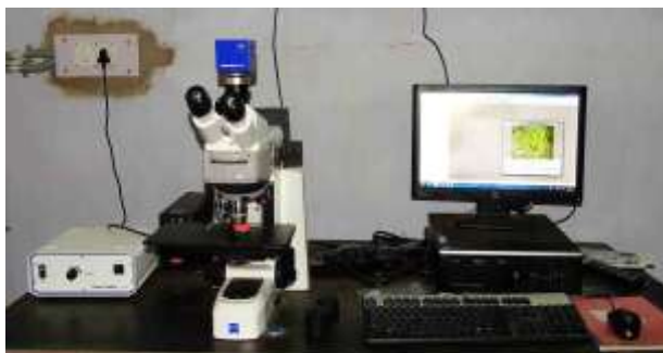
Fig. B.13 Optical microscope for measuring weld area
