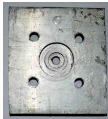
Fig. B.5 Aluminum backing plate
