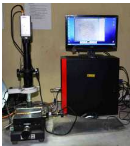
Fig. B.7 Optical microscope for measuring weld area
