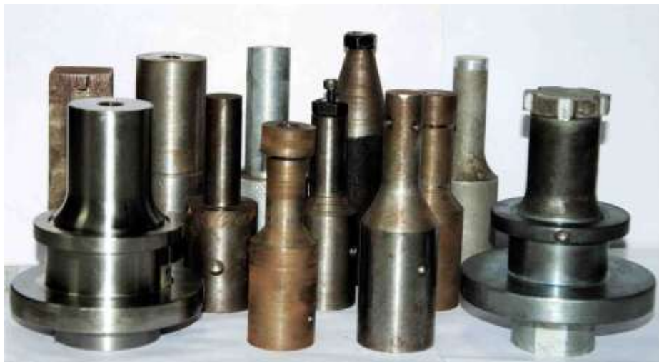
Fig. 3.17 Manufactured various spot welding horns and booster
