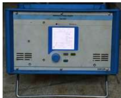
Fig. B.9 Charge amplifier
