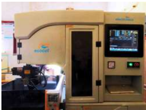
Fig. B.6 WEDM machine employed for making knurling features
