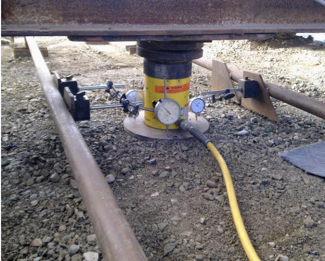
Fig. 5. Photograph of test installation prior to loading include reaction beam, load plate, hydraulic jack and three dial gauges.
