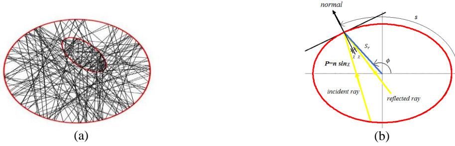
Fig. 1: (a) Cross-section of the SIF showing chaotic light rays. The core and cladding boundaries are both deformed from a circular shape, and are not co-axial, resulting in an asymmetric geometry. The rays bouncing around the fibre are a mixture of periodic and chaotic motions, and the classification can be made by illustrating the ray dynamics in the Poincaré surface of sections (SOSs). (b) The arc length s forms the horizontal axis, and P = n \sin\chi forms the vertical axis of the SOS. Each boundary in the step index fibre (SIF) cross-section has its own SOS.
