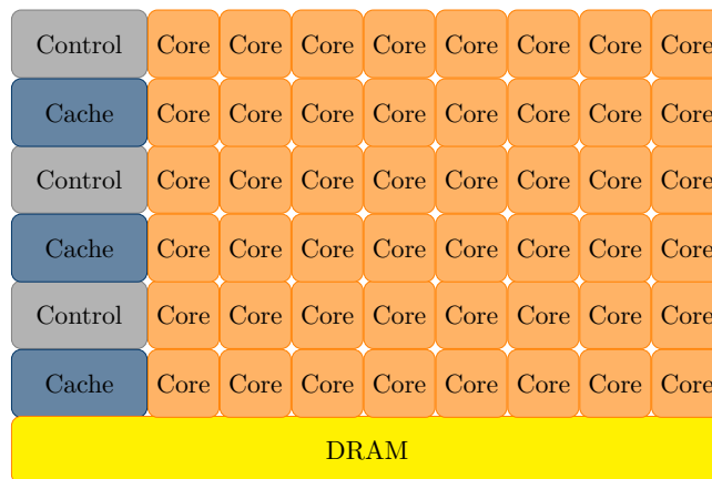
Figure 4: A schematic of a typical GPU, recreated from NVIDIA Corporation (2015).
