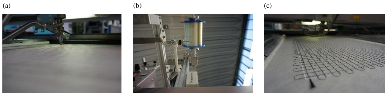
Figure 2. Modified embroidery machine at the STFI that consists on an embroidery needle (a) and auto-tracking of the optical fibre (b) to simultaneously process carbon and optical glass fibres on a PVA nonwoven substrate (c).
