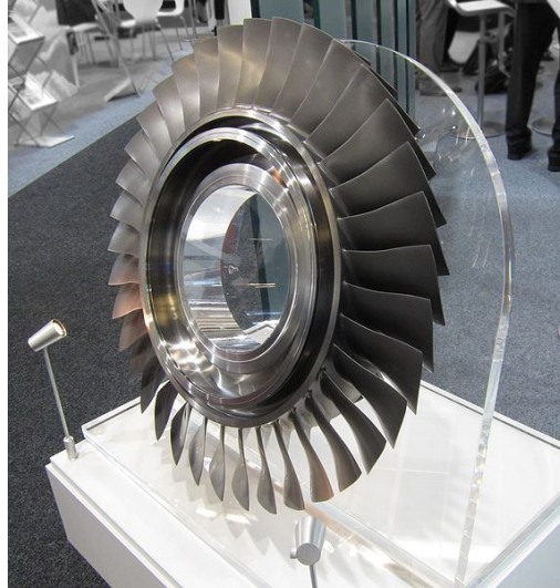
Figure 1: Example for a complex geometry: Blade integrated disc (Blisk). Source: Olivier Cleynen with creative common license CC BY-SA 3.0
