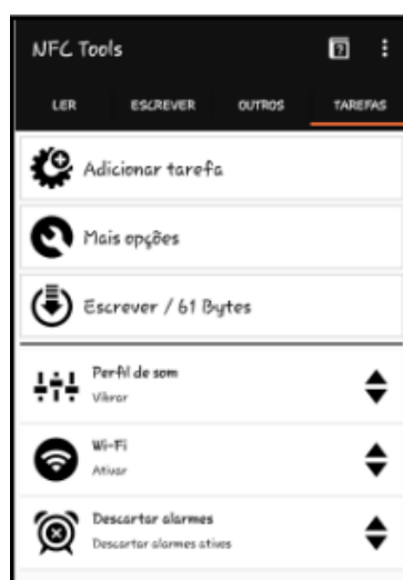
Figura 26 – Gravar tag com as tarefas de rede/som/alarme
