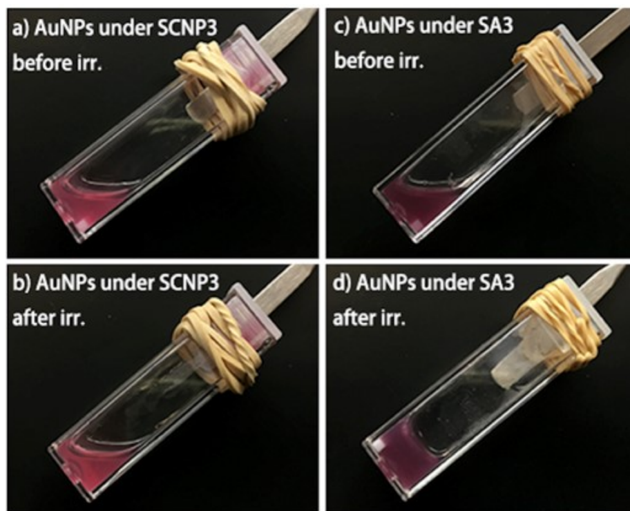
Figure 51. Photos for aqueous solutions of P(MEO 2 MA- co -MAA)- b -PEO- b -P(MEO 2 MA- co -MAA) (10 wt%) containing AuNPs (0.12 wt%) prepared using SCNP3 (a, b) and SA3 (c, d) respectively, showing the gelation only occurred in the latter solution after exposure to 635 nm red light at room temperature for 10 min.
