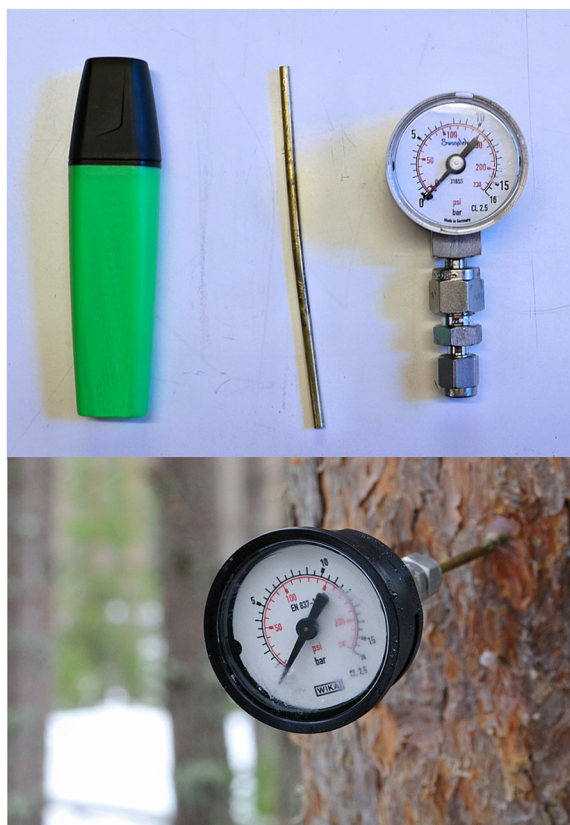
Figure 1. Components of the oleoresin exudation pressure (OEP) measuring system with Swagelok gauge (top) and the brass tube and WIKA pressure gauge attached to a pine tree at SMEAR II (bottom).
