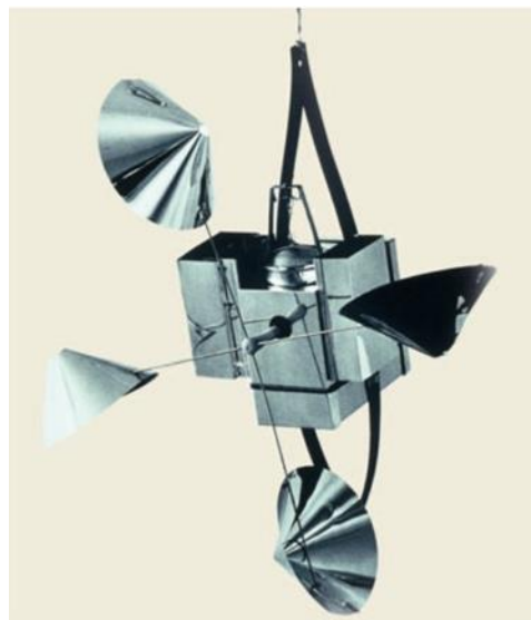
Figure 9. The first commercial model of the Vaisala RS11 radiosonde which entered the market in 1936.
