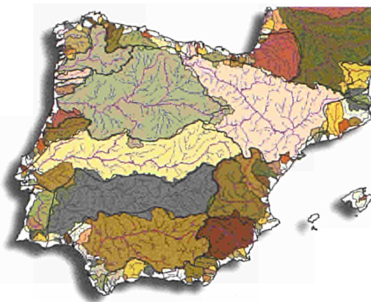
Major Iberian Catchments derived from a DEM with 1 km grid cell size.
