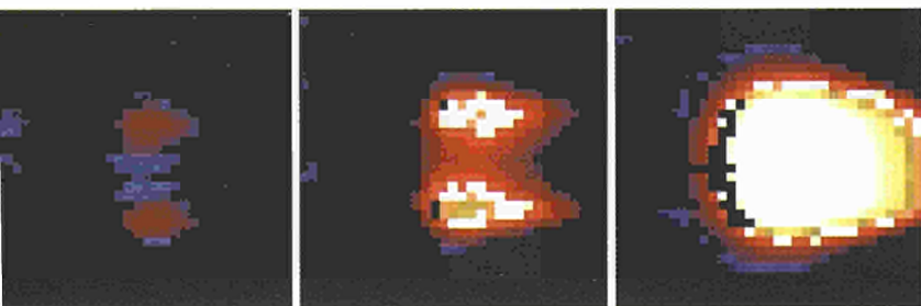
Example responses from a metal detector, scanning small cylinder, larger cylinder and washer (l to r) at a sweep speed of 0.5 m/s.
