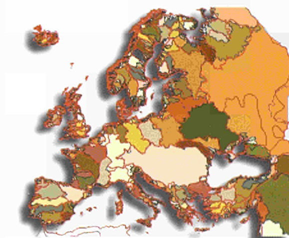
Major European Catchments derived from a DEM with 1 km grid cell size.
