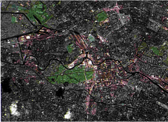
Fusion of IRS-1C LISS III and PAN data from Berlin, Germany; acquisition date 9-May-97; 5-m spatial resolution.
