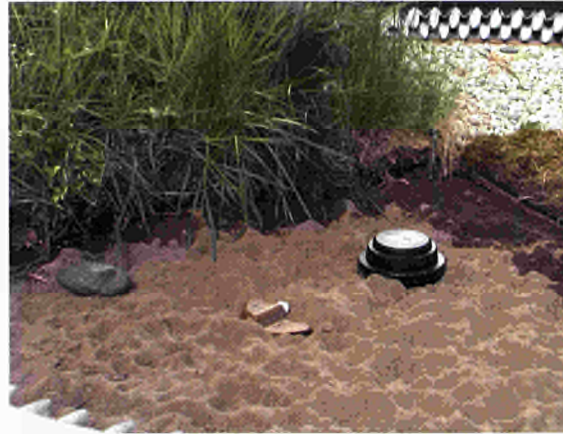
Mines placed on sand with defined surface roughness for measurement in the EMSL.
