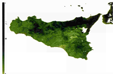
Results obtained with the Optimised Vegetation Normalised Index (OVNI) using data collected over Sicilia by the VEGETATION sensor.
