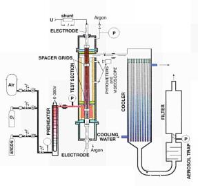
Figure 4.12: Schematic Diagram of the CODEX-AIT facility at AEKI Budapest for the Conduct of Core Degradation Experiments in Air.
