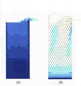
Figure 4.3: Computer simulated discharge of a steam and water mixture from a cylindrical pressure vessel via a horizontal outlet pipe, at two time intervals: (A) t=4 sec, (B) t=14 sec, showing complex twophase flow phenomena. Simulation made with the ISIS 'ATPF' pilot code.
