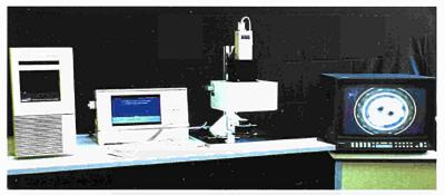
Figure 3.12: The verification station CIVES for metal cap seals comprising the image acquisition part with the special seal illuminator and the image archive unit.
