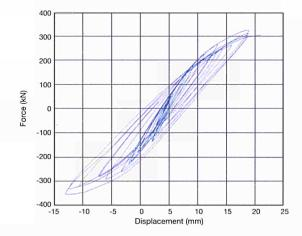
Figure 2.7b: Force-Displacement loops for cyclic test. Protection of the building is obtained through energy absorption in SMA device and structure. The hysteresis shows that the structure dissipates part of the energy.
