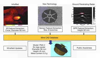
Figure 1.26: Example of target identification through the fusion of data from three different sensors with features extracted from a CAD database.
