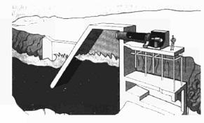
as computer simulations have indicated a significant potential for improvement in the plant efficiency. This implies a real-time blade-angle control according to one or more optimising strategies. JRC's task, within PIOWC, is to design and build the real-time control system for the turbine blade angle control of an innovative, variable pitch turbine that will allow the performance improvement in the existing OWC power plant.
