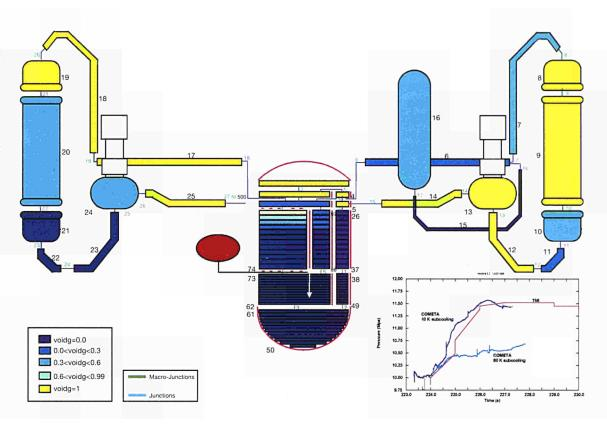
simulation of the TMI accident sequence [4.16]. A RELAP5/SCDAP calculation was performed in order to determine the conditions of the plant at the time of melt relocation. Figure 4.8 shows the void fraction distribution as calculated by this code and demonstrates that the vessel was full of water a the time of melt relocation.
