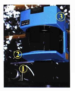
Figure 3.10: Laser Surveillance System constituted by a camera (1), an Infrared illuminator (2) and a laser range scanner (3).
