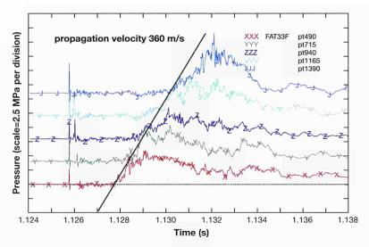
Figure 4.5: Upward propagation of the energetic event triggered in FARO test L-33; water depth 1.62 m, subcooling 122 K; pt=pressure transducer in water located on the wall of the test vessel at xxx mm from bottom as indicated; pressure scale=2.5 MPa per division.
