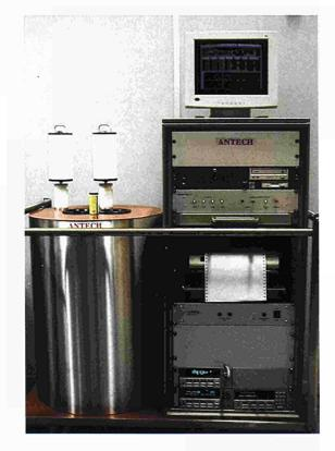
Figure 3.3: The new Small Sample Calorimeter (SSCAL) allows the characterisation of samples as small as 1g of plutonium at 0.2% precision.
