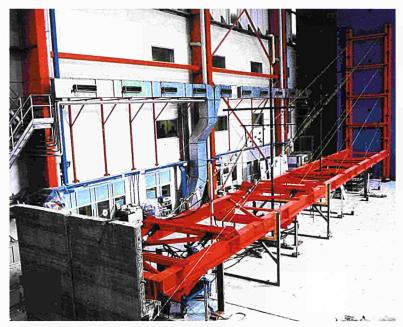
Figure 2.3: The Large-scale cable-stayed bridge mock-up at the ELSA Laboratory used to validate active vibration control devices.
