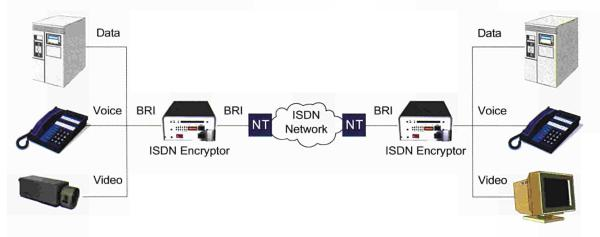
Figure 3.14: Description of the pilot secure communications system implemented between Ispra and the ESO headquarters at Luxembourg.
