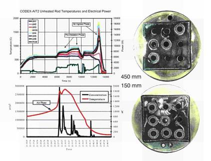
Figure 4.13: Air Ingress Experiment CODEX AIT2 Unheated Rod Temperature Histories, Aerosol Production in Air Phase and Cross-Sections showing Rod Degradation and Material Relocation.
