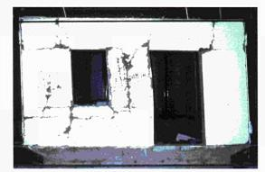
Figure 2.5: Top: Increased strength and ductility of the reinforced infill with openings (red curve) when compared to the plain one (blue curve). Bottom: Final state of the reinforced infill (the complete collapse of the plain infill is visible in the background).
