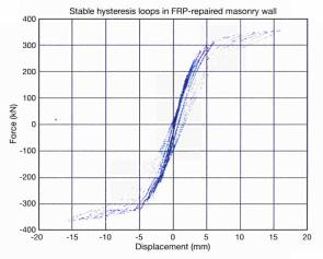
Figure 2.7d: Force-Displacement loops of the masonry wall protected with fibre composite material. The structure remains intact.
