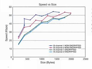
Figure 3.15: ISDN Monitoring –Measured data throughput and speed as a function of packet data size, and presence of encrypting devices.
