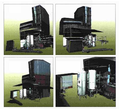
Figure 1.19: 3D Reconstruction of an outdoor industrial plant – the figure shows three snapshots of the final 3D reconstructed model as seen from three different positions and a close-up snapshot of the highly detailed 3D model of the pipe work.
