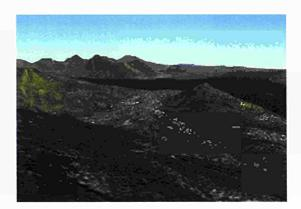
Figure 1.3: A virtual image generated from a digital elevation model and satellite image of the Lago Maggiore Region. The simulated view is calculated looking from Monte Zeda across the lake towards Laveno.
