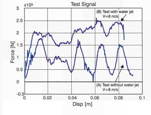
Figure 2.17: (A) Conventional crash energy absorbers exhibit deceleration peaks in regular intervals which would endanger the passengers' safety; (B) The test with the liquid water jet energy absorber shows a progressive crash energy absorption without harmful deceleration peaks.
