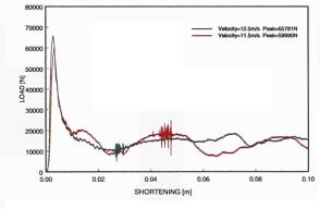
Figure 2.16: Load/Shortening curves of high strength steel longitudinal beams
