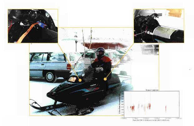
Figure 6.21: Cold Climate technology: Human-machine interface measurements reveal interesting results. The seat-pressure sensor (upper corner) gives information about the driver position. Accelerating measurements (lower corner) can exceed 2 G, a possible explanation for frequent bone-fatigue fractures observed with snow-mobile drivers.
