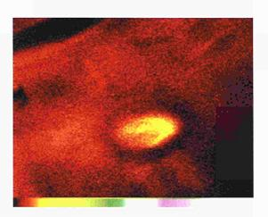
Figure 1.29: Infrared image of a mine totally covered by the sand: The measurement was performed after heating up the sand.
