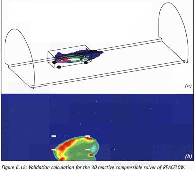
(a) The domain is a 20m section of a two-lane road tunnel, with a single stationary car. The simulation is of an explosion in a hypothetical hydrogen cloud around the car: the outline of the tunnel domain together with iso-surface plots of the hydrogen concentration, showing surfaces with hydrogen concen-trations of 8% (blue), 15% (green), and 29% (red) volume fraction.
