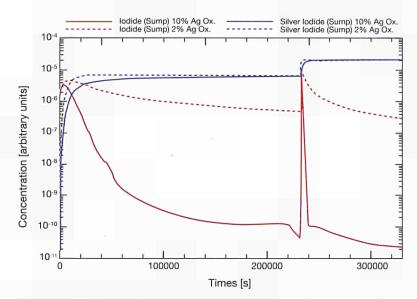
Figure 4.11: IMPAIR3 calculation of sump iodine in Phebus FPT1, showing non-volatile silver iodide (top curves) as the dominant species.
