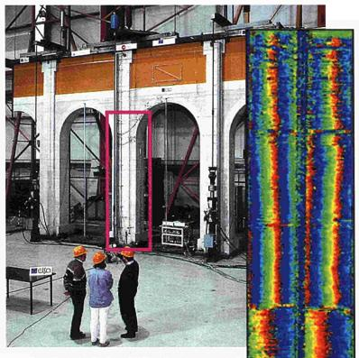
Figure 2.10: Application of DMS to the measurement of rotation of a column of the full-scale model of St Vincente de Fora under seismic testing. The column was prepared with stripe patterned paper and imaged on to a CCD camera array, forming moiré fringes. These were analysed in real time to display the movements of the column blocks.
