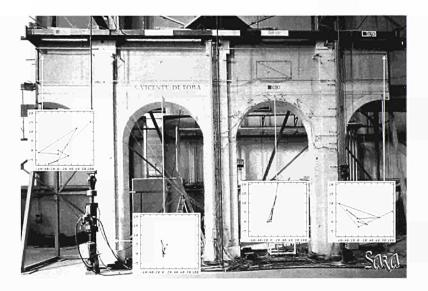
Figure 2.9: Photogrammetry used to monitor a model of the Portuguese Monastery Sāo Vicente de Fora during PSD testing: During the seismic experiment the actuator connected to the upper right part of the building pushes and pulls the building until structural damage occurs.
