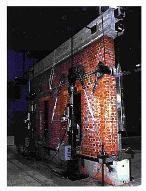
Figure 2.7a: Masonry wall protected with Shape Memory Alloy devices at the ELSA laboratory. In applications as in the bell tower of Trignano (RE, Italy) or the tympanum of St. Francis Basilica, Assisi, the Shape Memory Alloy devices are installed maintaining the architectural appearances of the buildings (V. Renda).
