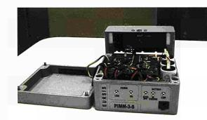
Figure 3.2: A prototype pressure instrument module was designed for accurate in-field measurement of liquid mass and volume in tanks (PIMM).
