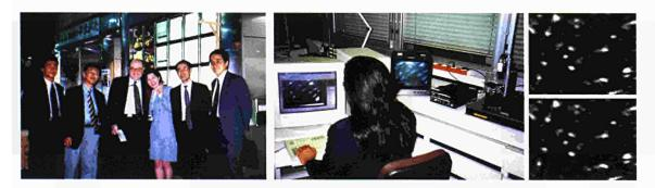
Figure 3.6: Left: Meeting in Tokyo with Hitachi and Toshiba Colleagues while negotiating the Contract on MOX Fuel Sealing Systems. Middle: Laboratory test mounting for the Identification of Surface Textures by "Speckle" Effect, using a Laser Diode. Right: Two "measures" of the same area are shown.
