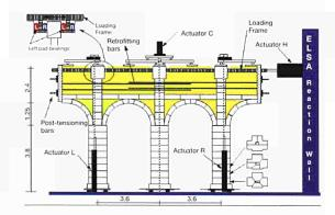
Figure 2.8: S. Vicente model - Test set-up and location of the continuous-bond retrofitting bars.
