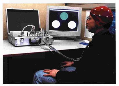
Figure 1.13: Portable EEG system. In this picture, the user holds a cap with integrated electrodes. The cap is connected to the dedicated hardware (left). The computer screen shows how the user receives biofeedback in real time. There are three buttons, one for each mental task to be recognised. A button lights up when the current EEG sample is classified as belonging to the corresponding mental task.
