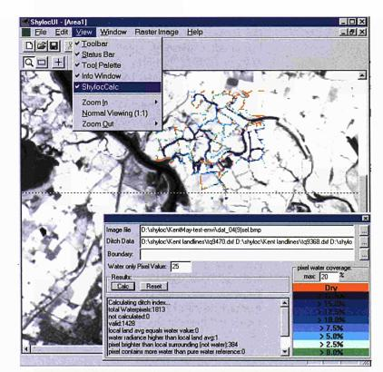
Figure 6.19: The SHYLOC user interface (main screen) and colour-coded view of percentage of the ditch network that is full of water (inset screen). The main screen shows the status of the stream network in the Elmley Marshes, N. Kent Marshes, England in February 1998.
