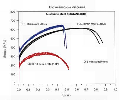
Figure 4.9: Stress-strain curves to be considered when assessing the reactor vessel structural safety under severe accident conditions. The measurements show a drastic effect of the speed of deformation (strain rate) and of temperature on the behaviour of the austenitic steel as used in the Reactor Pressure Vessels of the Upper Internal Structure.
