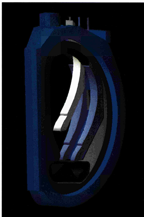
Figure 2.47. Simulation of withdrawal of Blanket segments from one sector of the vacuum vessel of ITER.
