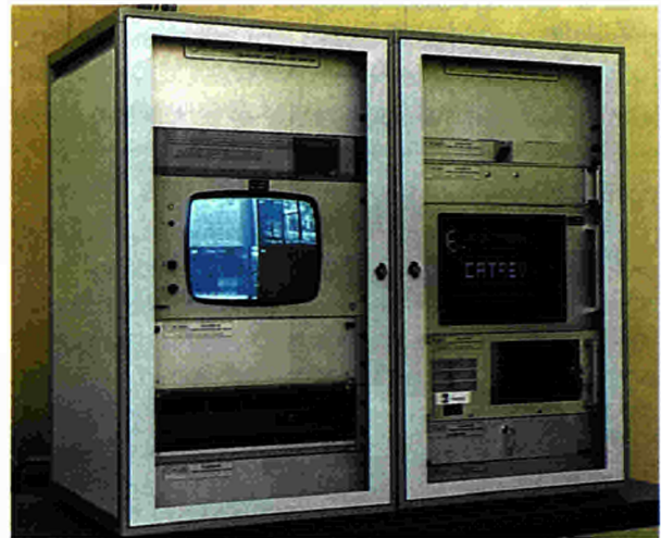
Figure 4.12. Review station for video surveillance.
