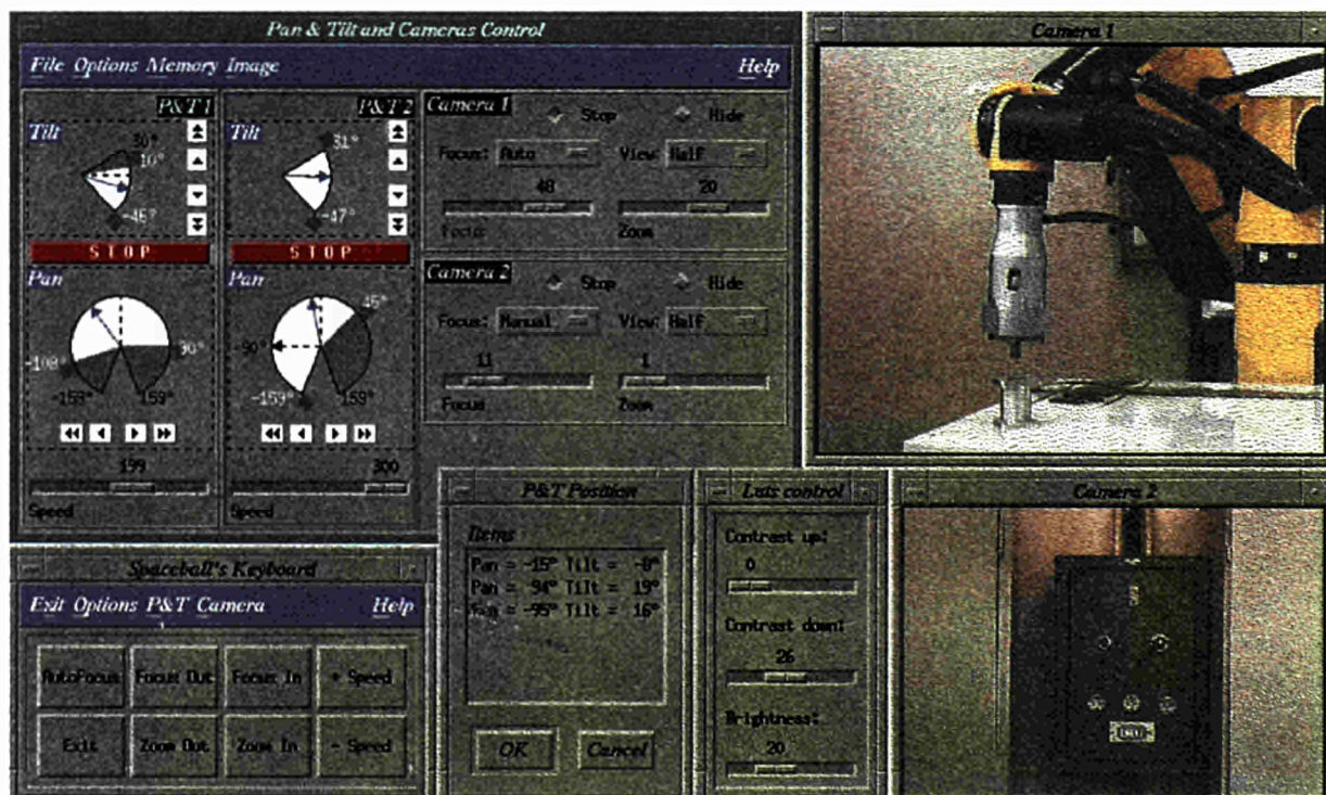
Figure 2.43. Remote Surveillance System: Human-Computer Interface allowing for full interactive control of TV cameras, pan-and-tilt units and motorised lenses.
