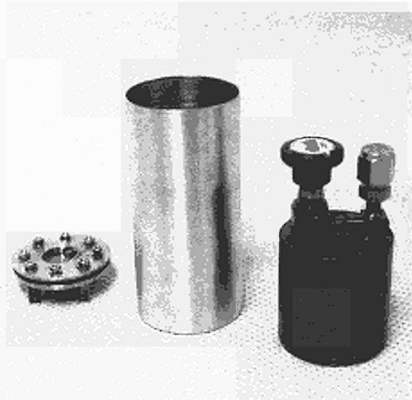
Fig.234: Amersham Mark IV transport U-bed with calorimeter secondary confinement.
