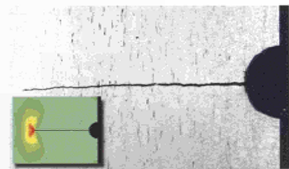
▲ Stresses at the crack tip of a crack grown in a component wall grown by thermal fatigue from a starter notch.
