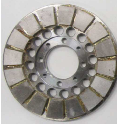
Figure 8.7: The rotor with holes with the trapezoidal aluminum of the studied AFPMSM.
