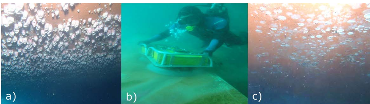
Figure 1: a) Marine fouling on the flat bottom of a tanker vessel b) Diver cleaning the hull using a portable brush cart c) Flat bottom after hull cleaning
