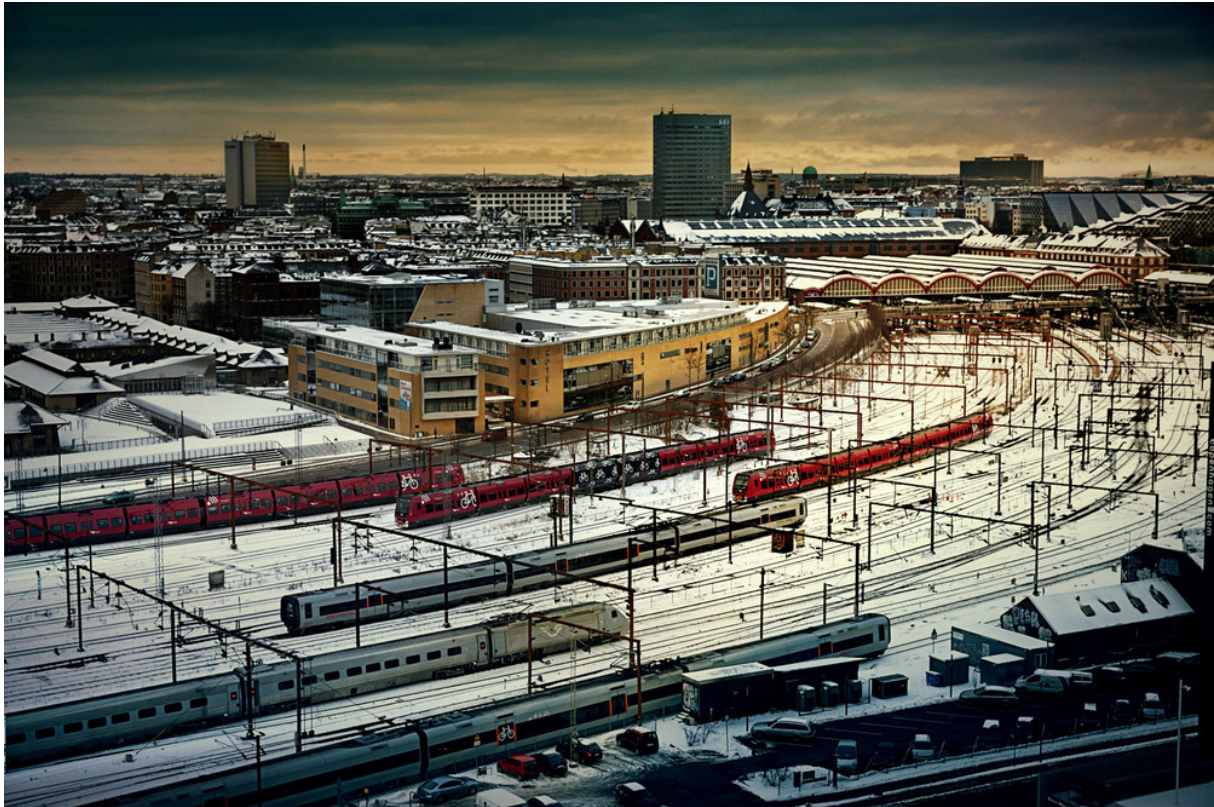
Figure 2.3: Impressions of the rolling stock operation just south of København H station, Thursday 2012-12-13 at 12:20. The red DSB S-tog train unit to the left is heading south on the main line tracks towards Dybbølsbro station. The middle, red train unit is in the process of being shunted from the depot to København H station to enter revenue train service. Note the special livery to advertise the then new flexible space sections in the middle of the train unit. The right, red train unit is heading north on the main tracks towards platforms 9/10 at København H [73].
