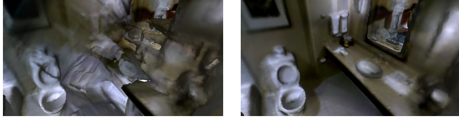
Figure 4.6: Fatal tracking failure prevented. Left: the mirror causes a purely geometric camera tracking approach to fail, the reconstructed volume turning out unrecognisable. Right: tracking succeeds and the bathroom is correctly mapped thanks to the employment of semantic clues during camera pose estimation.
