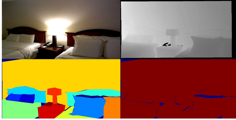
Figure 3.3: Labelled frame from the hotel room sequence of the Sun3D dataset [123]. From top left in clockwise order: RGB frame, depth frame, score map and category map. The score map has been drawn in false colours to increase visibility (blue is the minimum value while red is the maximum). In the category map each colour represents a different object instance.
