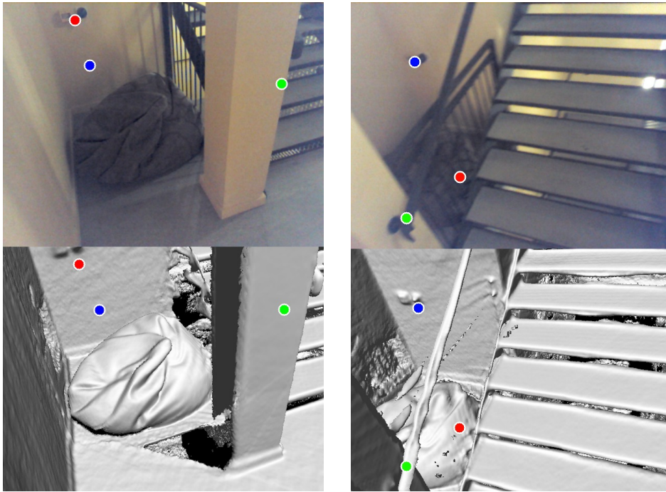
Figure 6.9: From certain angles in the Stairs scene, the relocaliser is able to rely on points in the scene that can be identified unambiguously to estimate the pose.
