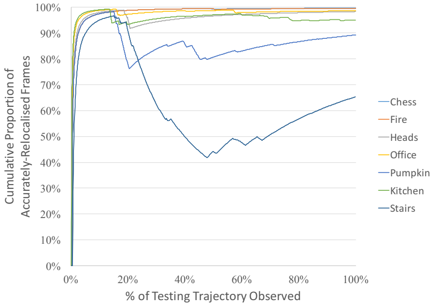
Figure 6.3: The performance of our approach for tracking loss recovery (Subsection 6.4.2). Filling the leaves of a forest pre-trained on Office frame-by-frame directly from the testing sequence, we are able to start relocalising almost immediately in new scenes. This makes our approach highly practical in interactive scenarios such as 3D reconstruction.
