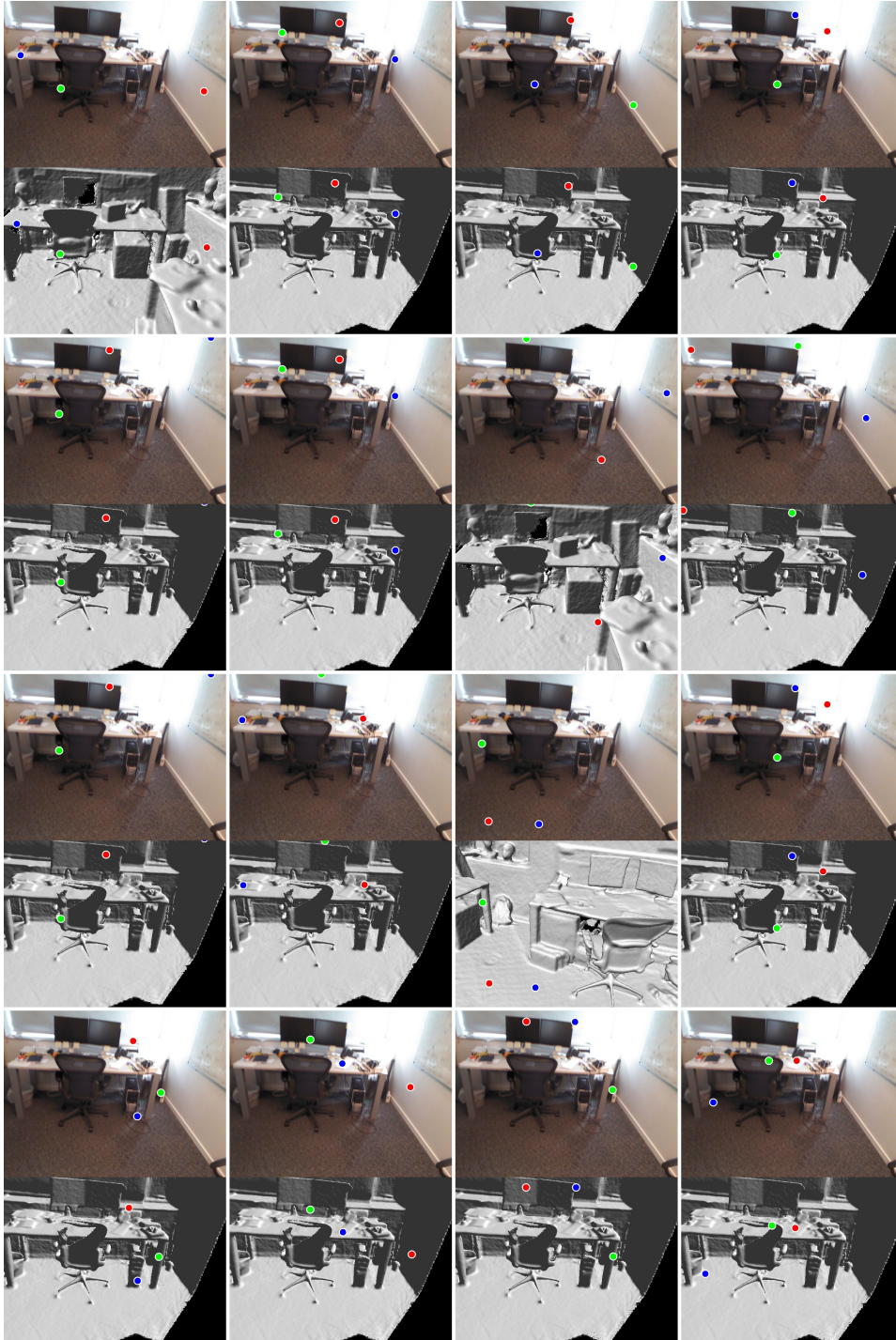
Figure 6.7: The top 16 pose candidates (left-to-right, top-to-bottom) corresponding to the failure case on the Office scene shown in Figure 6.6d. The coloured points indicate the 2D-to-3D correspondences that are used to generate the initial pose hypotheses. Note that whilst the top candidate selected by RANSAC relocalises the camera to face the wrong desk, any of the next five candidates would have relocalised the camera correctly.
