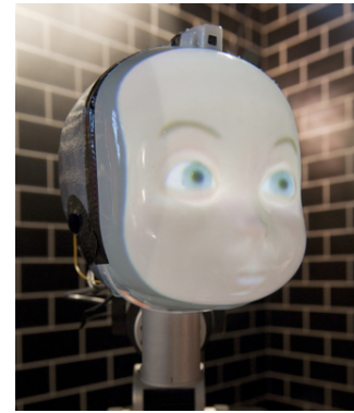
Figure 1: the LightHead robot face, mounted on a robot arm (Jennie Hills, Science Museum, London).
