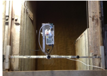
(b) Camera mounted above the flume on the horizontal frame, looking down onto the seeding particles.
