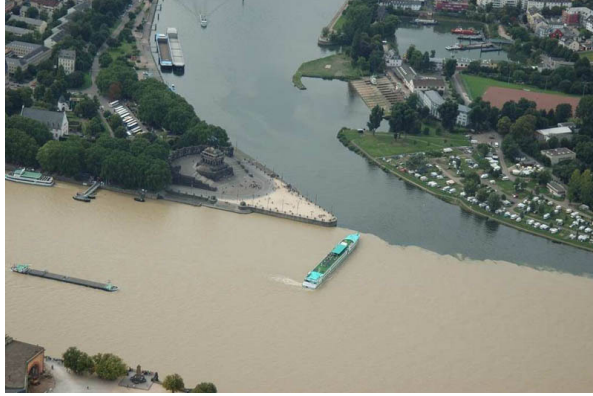
Figure 1.1: Confluence of the Mosel and Rhine (Germany). The difference in water color (caused by difference in sediment load) visualises the (central) mixing layer between both confluent flows.
