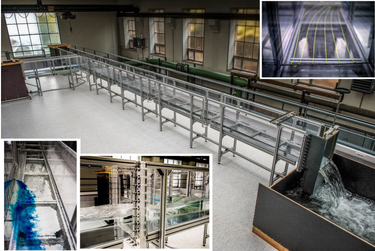
Figure 4.1: Impression of the confluence flume, applied for confluence research. Blue dye has been applied to outline the separation zone, yellow wires are applied in the tributary to illustrate the streamline curvature.
