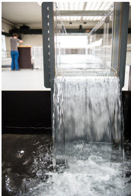
Figure 4.5: Downstream weir in completely lowered position.
