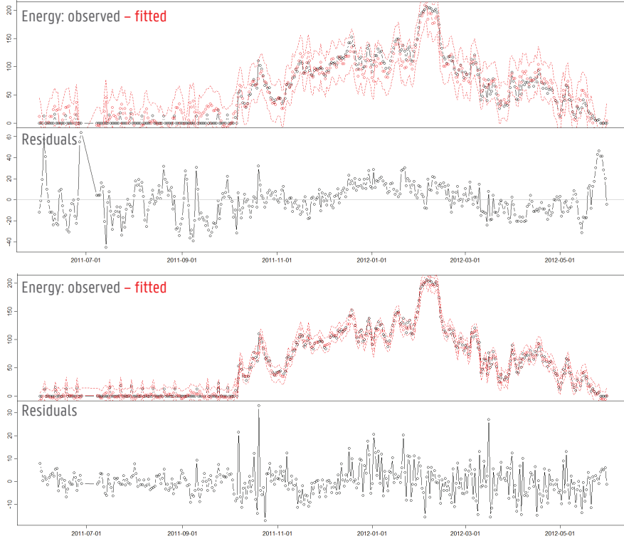
Figure 5-67: Time Series Plots of the energy use and residuals , for the LM(top) and LMCIS-model (bottom)
