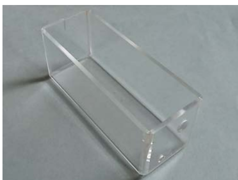
Figure 1. Custom made transparent Plexiglass® growth monitoring chamber
