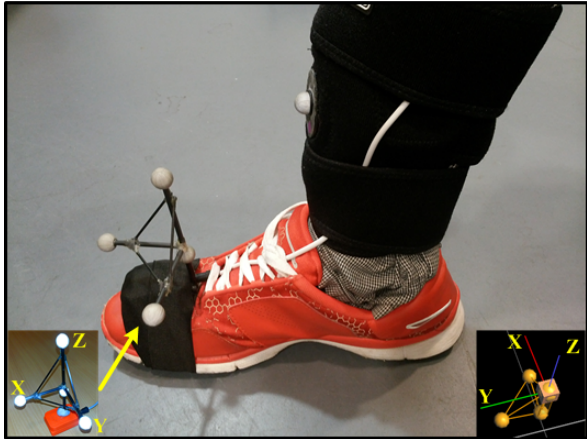
Figure 1 Sensor attachment and Vicon marker placement
