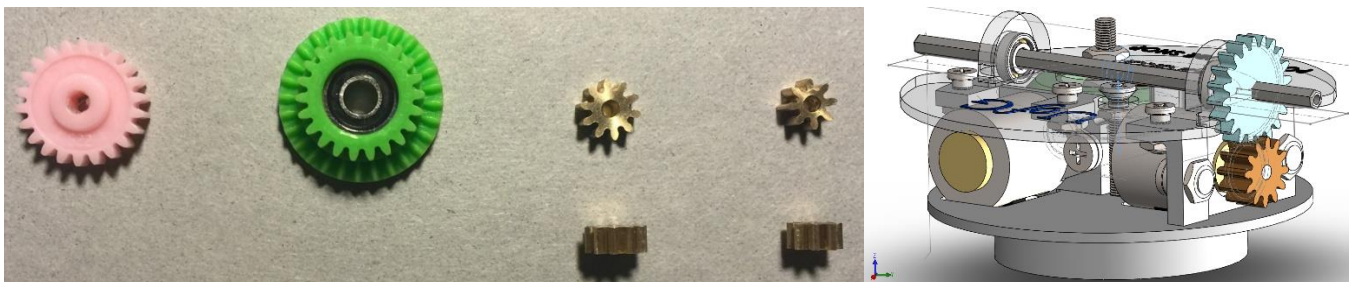
Figure 10. 22-Tooth Spur Gear, Crown-Spur Double Gear (28T-22T), 10-Tooth Pinion Gear 2, 8-Tooth Pinion
