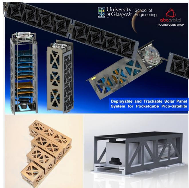
Figure 1. Top: Poster – 3P PQ & Solar Panel System Below Left: Photos- the 1P,1.5P,2P,3P PQ Skeletons Below Right: Illustration- PQ Launcher with a 2P PQ
