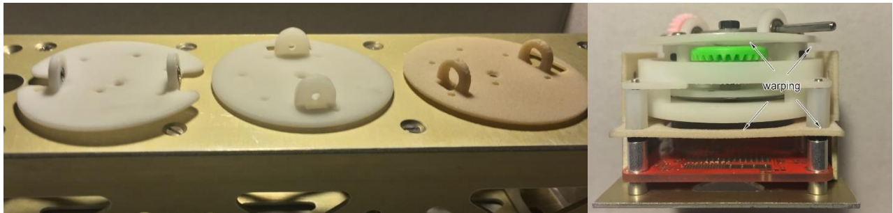
Figure 34. Unwanted warping is a common problem of 3D printing parts with thin-panel structure
