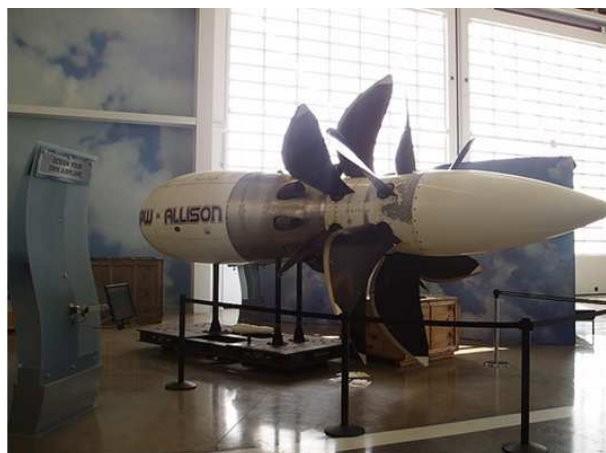
FIGURE 3.4: Pratt & Whitney 578 DX developed with Allison Engine Company and Hamilton Standard 15
