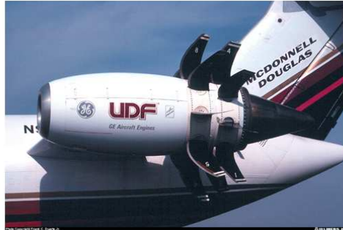
FIGURE 3.2: GE-36 UDF technology demonstration mounted on a modified MD-80 15
