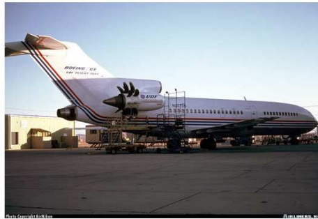
FIGURE 3.3: UDF engine on a Boeing 727 15
