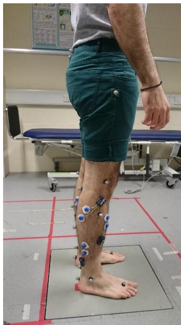
Figure 5.6. Side view of surface EMG electrode application on the gastrocnemius lateralis, gastrocnemius medialis, soleus and tibialis anterior muscles of a volunteer during Gait Laboratory experiments.
