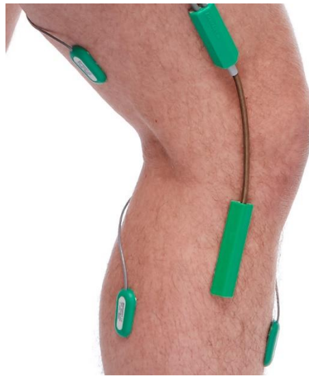
Figure 3.3. A Biometrics Ltd goniometer. Two green sections are attached to the upper and lower part of the knee with double sided tape. The flex of the metal braded connection measures the acute angle between the two green sections. Image taken from [88].
