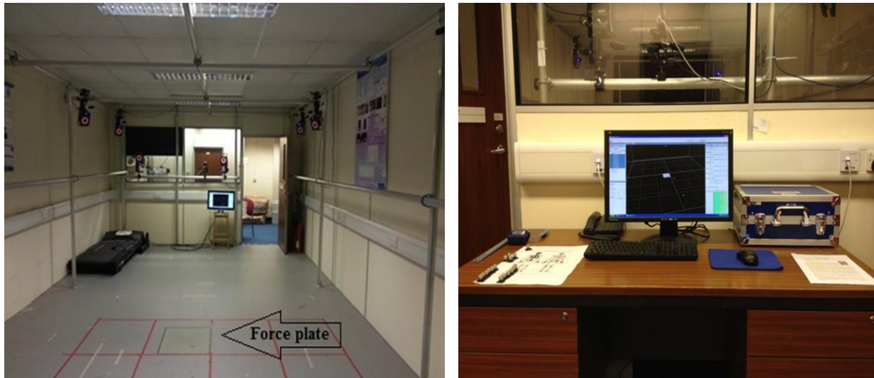
Figure 3.5. Gait Laboratory; rear view of the actual lab where the motion capture area is located. It is displaying the other six infra-red motion capture cameras. The same AMTI force plate is indicated by the arrow in the figure to the left. The monitor next to the door shows a live reconstruction of the 3D space experiments conducted in the laboratory and is synchronised with the monitor in the control room in the figure to the right, where a 2D grid represents the floor and a grey square represents the force plate.
