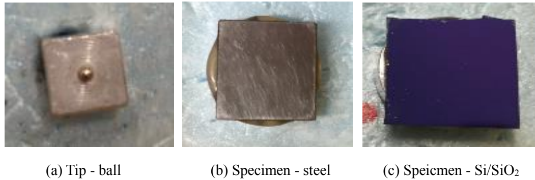
(i) Ball-on-flat configuration
