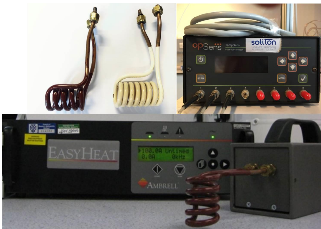
Figure 2.2 Image of coils (upper left), fibre optics signal conditioner (upper right) and induction heating units (bottom)
