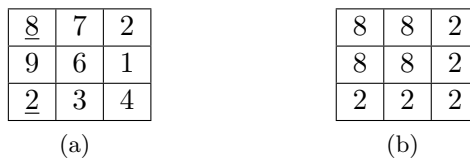
Figure 1.3: Pixel aggregation: (a) Image with seeds underlined, (b) segmentation result with \tau = 3 .
