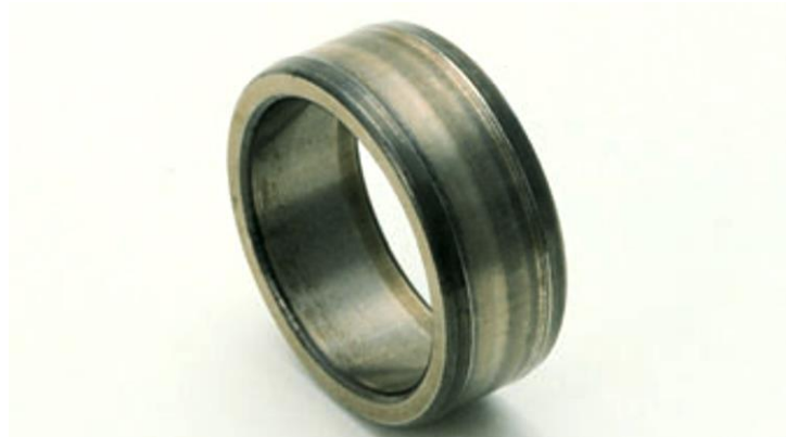
Figure 2-6 Example of bearing wear caused by abrasive particles [111]
