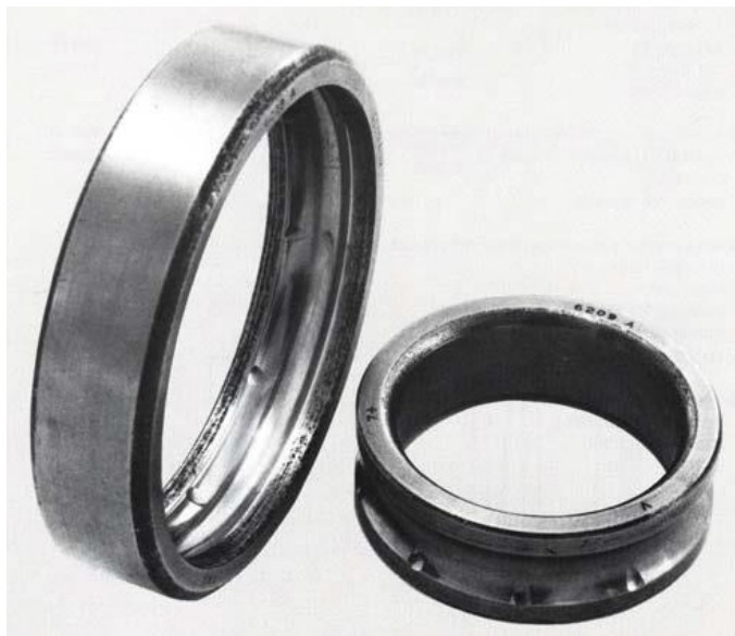
Figure 2-7 Bearing surface indentation [111]
