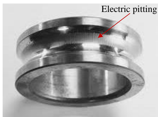
Figure 2-11 Electric pitting in bearing surface [107]
