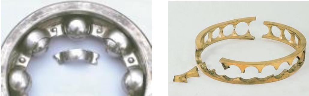
Figure 2-14 Bearing cage damage [107]
