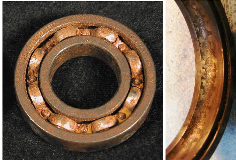
Figure 2-10 Deep-seated rust on the bearing surface [14, 111]
