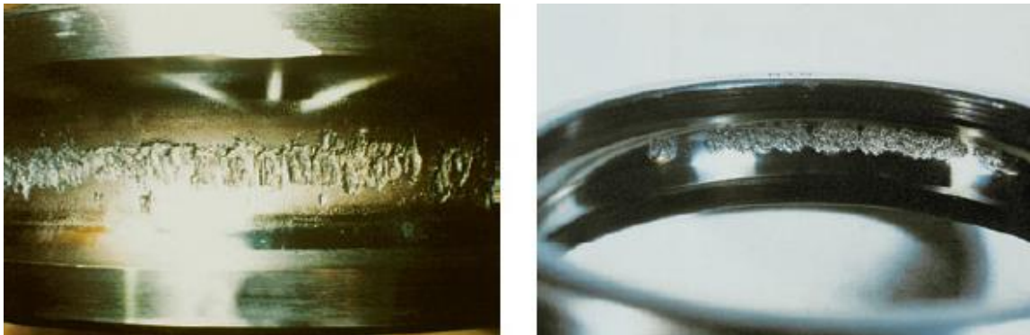
Figure 2-12 Spalling or flaking in bearing surface [111]
