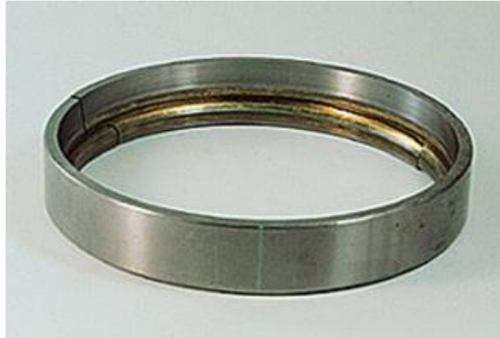
Figure 2-13 Showing an example of a crack defect in the bearing surface [111]
