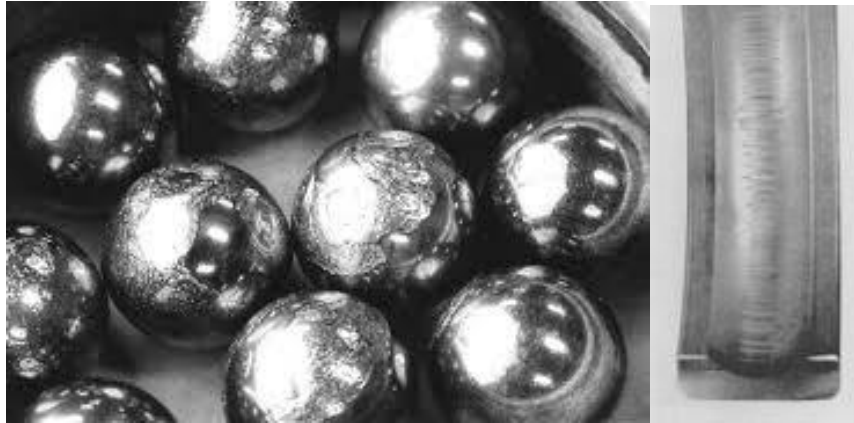
Figure 2-8 Bearing surface smearing [111]
