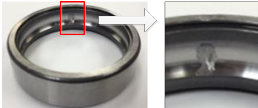
Fig. 16 Photographs of the test bearing with a small seeded outer race defect
