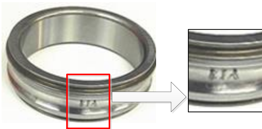
Fig. 21 Inner race defect on bearing
