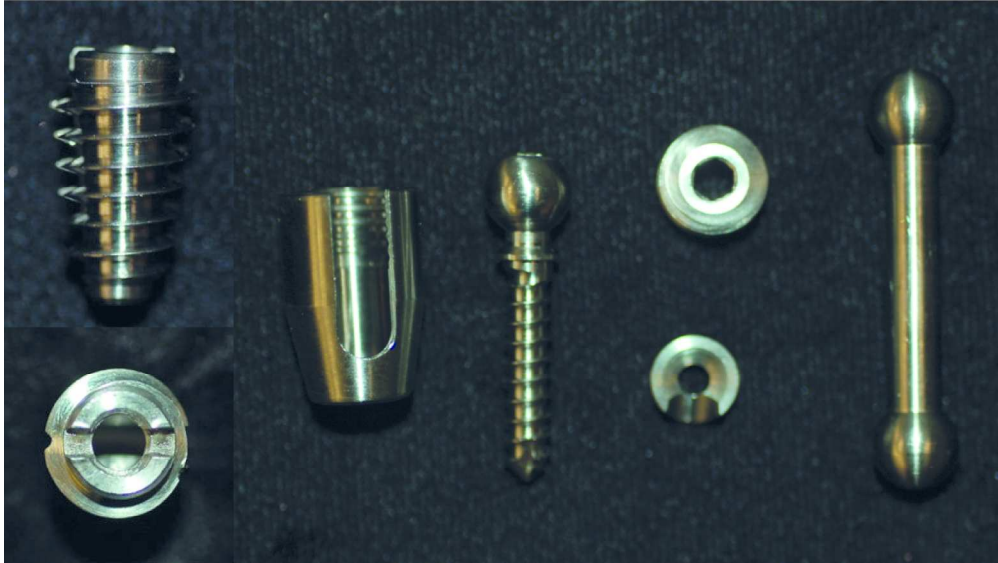
Fig 1. Photographs of the intervertebral distraction bolt (top: side view, bottom: view from on top) and the components of the pedicle-screw rod fixation system: clamp, 3.5mm polyaxial screw, washer (bottom, notice the dipped inner circle and the indentation of the rim to accommodate the dumbbell-shaped rod), nut (top) and dumbbell-shaped connecting rod (from left to right).
